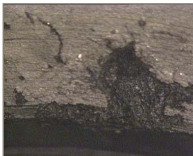
Pitting on filter end-cap
