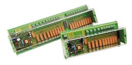
The 2000IO expander can increase the digital IO providing the option for greater remote operation of the programmer and expands the 2604 controller logic capability.
