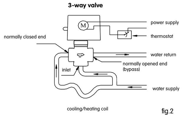
**3-way valve with clamp-on changeover switch**
