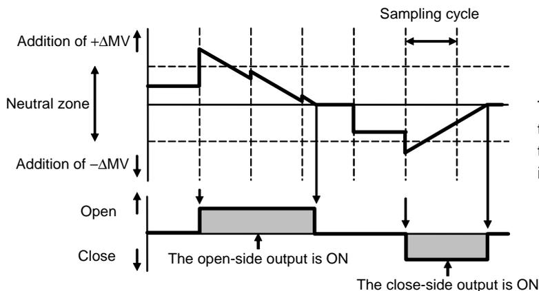
The controller does not output the  $\Delta MV$  to a control motor when the PID computed output value is within the neutral zone.
