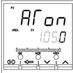
Set the upper limit values of the valve position (Feedback resistance input) which is opened and closed by output ON/OFF at Autotuning (AT) execution.
