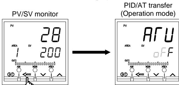
Press and hold the Shift key for 2 seconds
