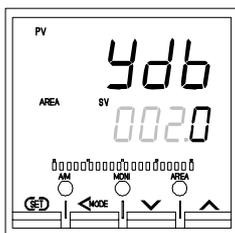
Set the output OFF zone between open-side and close-side outputs.
