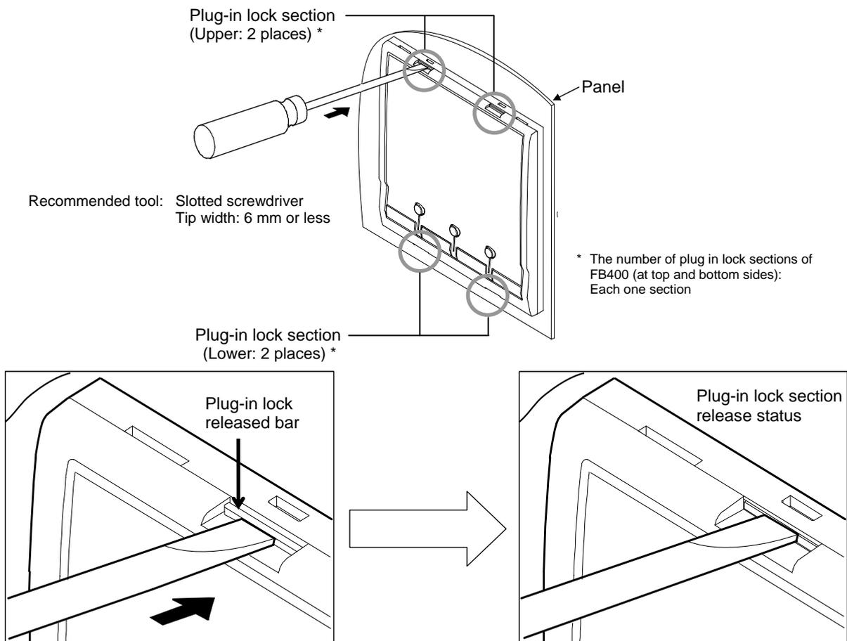
2. Insert the screwdriver in the case lock section as shown in the following figure, and then lightly turn the screwdriver to release the case lock section. The case lock section is released.
