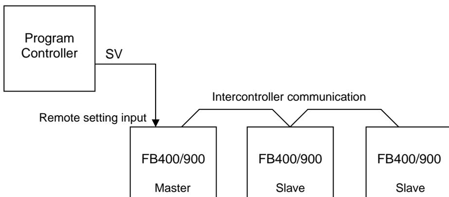
The master SV values continuously change gradually, the same as the program controller Set value (SV), but since there is a time lag due to Intercontroller communication, the slave SV changes in a stepped state.
