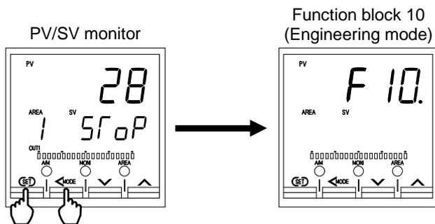
Press the Shift key while pressing the SET key for 2 seconds
