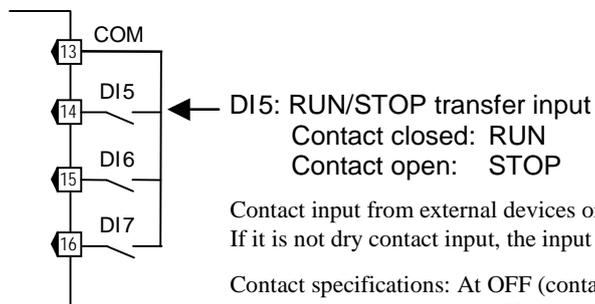
Contact input from external devices or equipment should be dry contact input. If it is not dry contact input, the input should have meet the specifications below.
