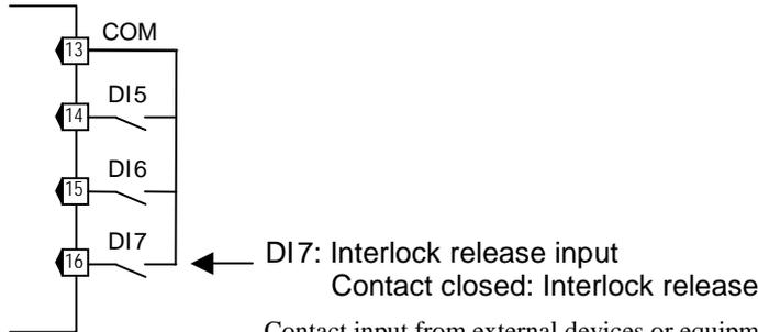
Contact input from external devices or equipment should be dry contact input. If it is not dry contact input, the input should have meet the specifications below.
