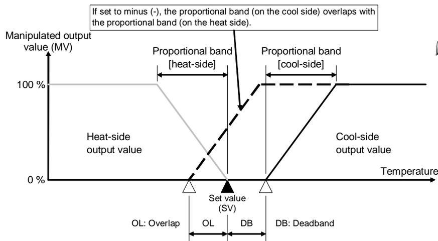
The diagram is an example when setting 0.0 to the Overlap/Deadband reference point. For Overlap/Deadband reference point, refer to P. 7-144.
