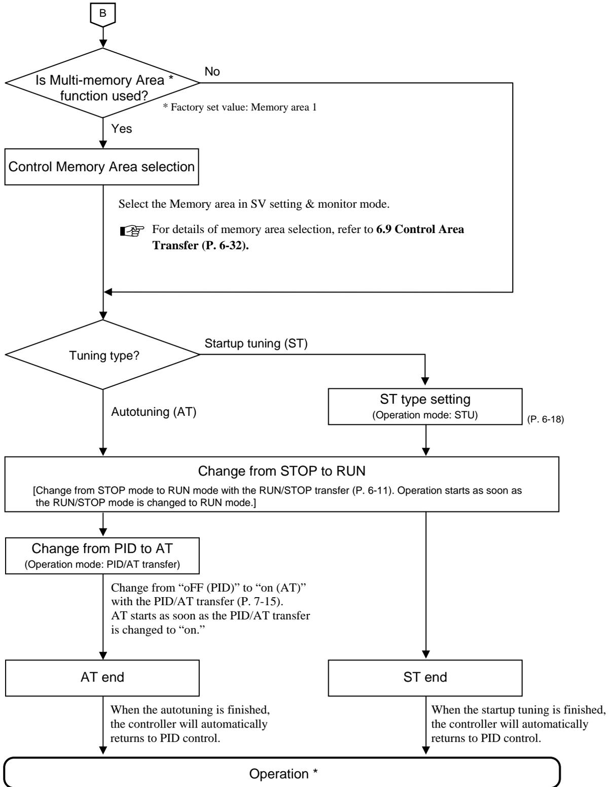
\* Adjust the PID constants manually when the optimum PID constants cannot be computed by Autotuning for characteristic variations of the controlled system (refer to page 6-9).
