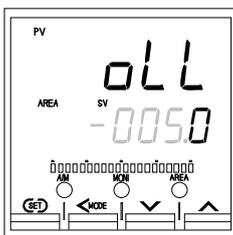
Set the low-limit value of the valve position.
