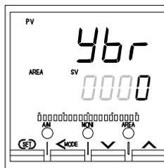
Set the action at Feedback resistance (FBR) input error.
