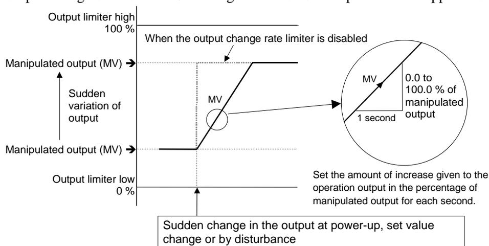
The output changes at specific rates set by Output change rate limiter (up) even under the situations where a sudden output change would occur without Output change rate limiter function. There is also independent Output change rate limiter (down).
