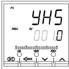
Set the differential gap of open-side and close-side outputs.
