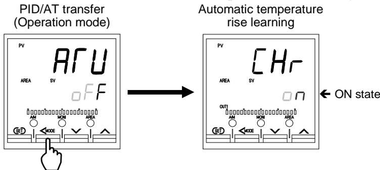
3. When the UP key is pressed, it switches from “oFF” to “on.” In addition, since the shipping value is “on,” when executing Automatic temperature rise leaning, it can be used as is.
