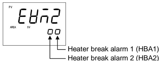
This screen is not displayed when set the CT assignment to “0: None.”
