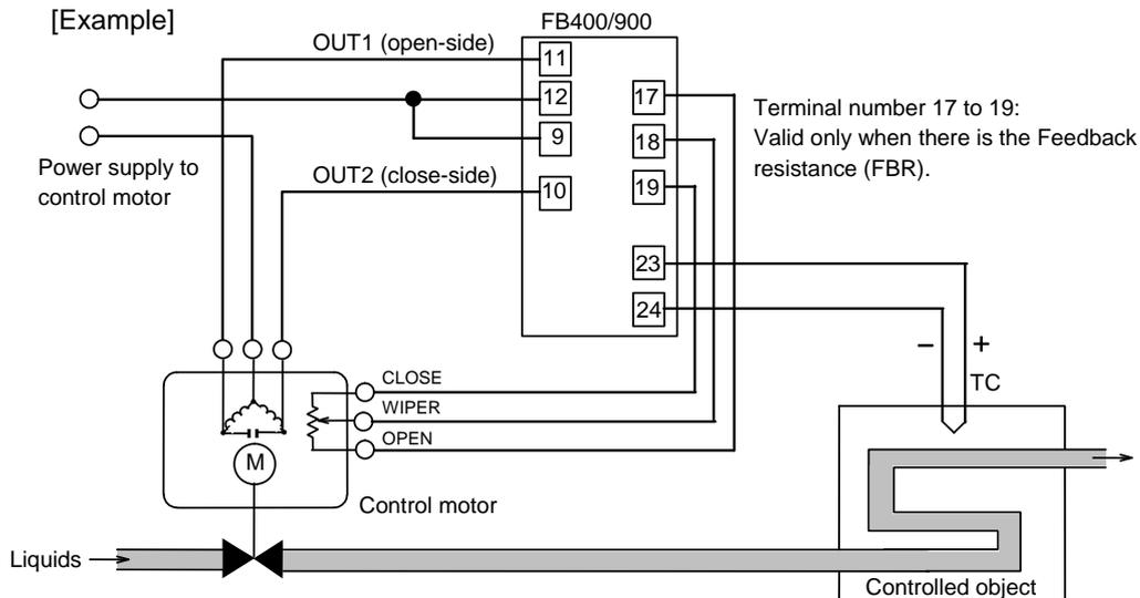
The details of setting differ depending on the presence or absence of Feedback resistance (FBR) input.
