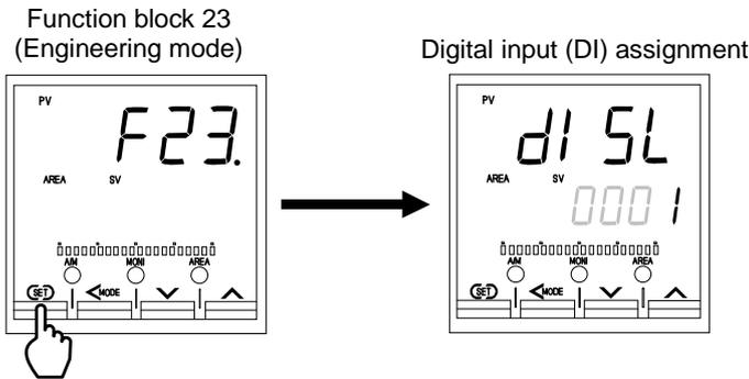
5. Set the Digital input (DI) assignment by pressing the UP or DOWN keys.
