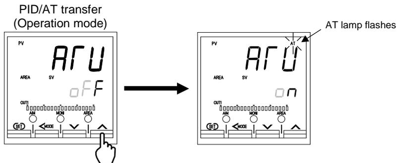
3. When the Autotuning (AT) is finished, the control will automatically returns to PID control. At this time, the AT lamp turns off.
