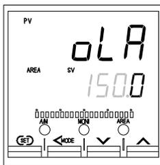
Set the Integrated output limiter which integrates the output and sets the output to OFF when the result reached the set value when an open-side (or close-side) output is outputted continuously.
