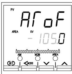
Set the lower limit values of the valve position (Feedback resistance input) which is opened and closed by output ON/OFF at Autotuning (AT) execution.
