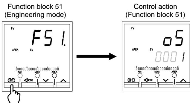
5. Press the UP key to change the control action from “1: PID control (reverse action)” to “5: Position proportioning PID control (reverse action).” Then, press the SET key to store the new value.
