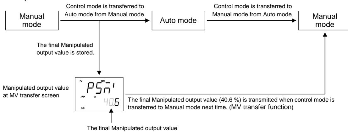
In addition, on this screen it is possible to manually change Manipulated output values (MV1 and MV2) in Auto mode. However, if they are changed in Auto mode, these manipulated output values thus changed are transferred when selected to the Manual mode next time.
