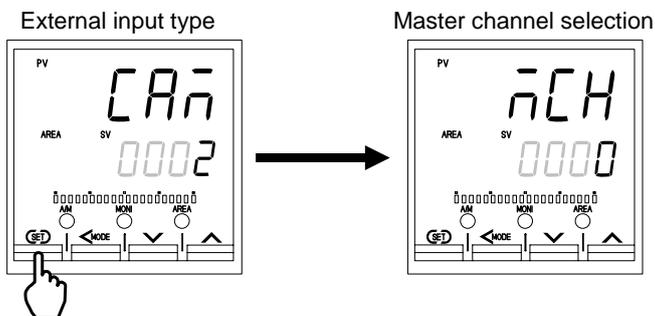
7. Press the UP key or DOWN key and set the address (value set by the Device address 2 screen) of the controller specified the ratio setting master. Set the Master channel to only the slave controller. No setting of the master controller is required.
