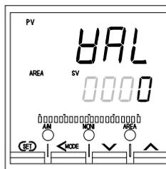
Set the action of open-side and close-side outputs at control STOP.
