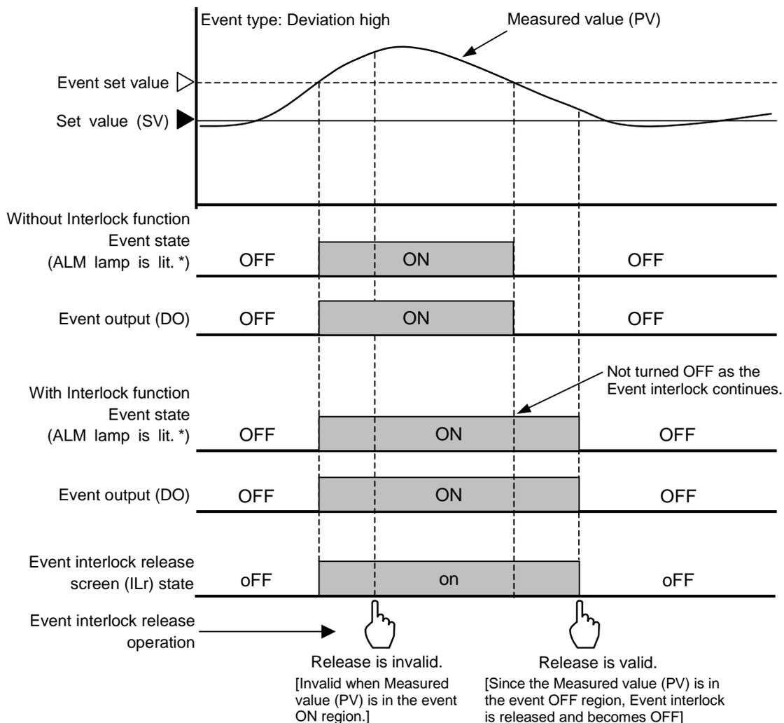
\* Set an alarm lamp lighting conditions to EV1 to EV4 in the Engineering mode. The alarm (ALM) lamp is lit through the OR operation of EV1 to EV4 each of which is set to "1: ALM lamp is lit". (Factory set value: ALM lamp is lit)
