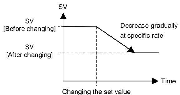
When the Setting change rate limiter is used, the SV will also ramp up or ramp down by the function at power-on and operation mode change from STOP to RUN.
