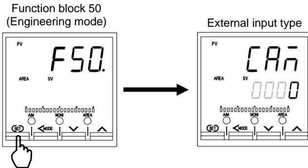
5. Select the External input type which needs to be changed by pressing the UP or DOWN key. Set "0" to the master controller and "2" to the slave controller.
