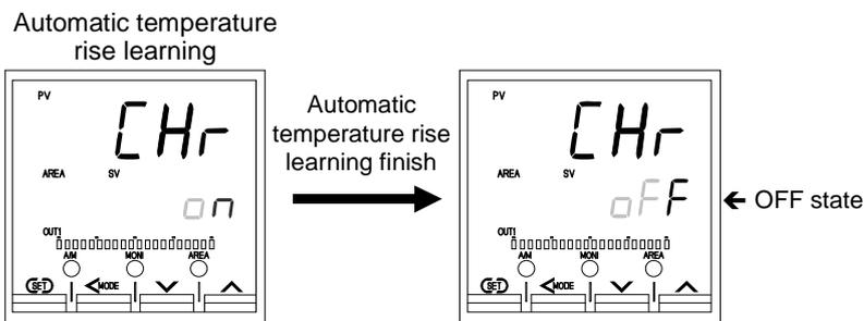
**At this point, the data necessary at Automatic temperature rise is only collected. Automatic temperature rise is not yet executed. Automatic temperature rise can be executed from the next startup.**
