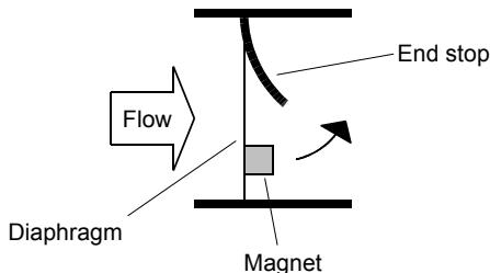
There is a plastic-coated magnet on the diaphragm. When there is a deflection, its magnetic field changes, and this is detected by a sensor outside the area of flow.
