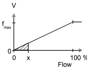
f<sub>max</sub> selectable in the range of up to 2000 Hz
