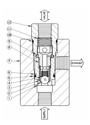
The **13QS40/41/80** is a two position, **6,000** PSI poppet operated <u>high flow exhaust</u> control valve assembly. It establishes flow from the Supply to Valve (inlet to outlet) connections to open a Surface Safety Valve (SSV or hydraulic Actuator) automatically with each application of operating pressure.
