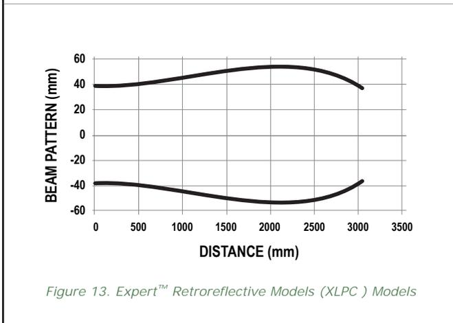
Figure 13. Expert™ Retroreflective Models (XLPC) Models
