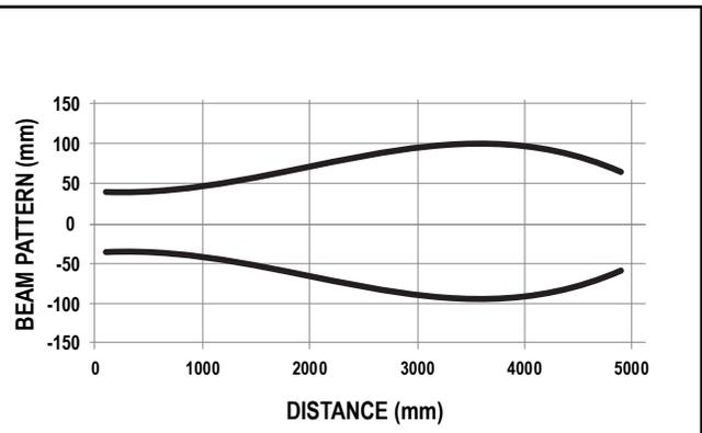
Figure 12. Fixed Gain Retroreflective (LP) Models
