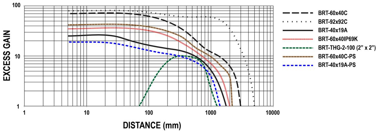
Figure 9. Fixed Gain Retroreflective Models (LP models)
