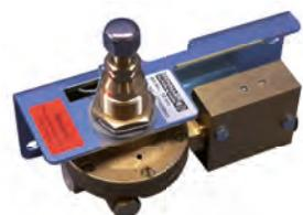
Pressure regulation unit (Illus. 8) The pressure regulation unit consists of a pressure regulator and a throttle block with an integrated air filter. The throttle block ensures that the drive air pressure in the VISATRON® oil mist detector does not increase to an excessively high level if the pressure regulator fails, (e.g. failure of diaphragm). The pressure regulation unit is delivered, pre-assembled and ready to operate, with its bracket.
