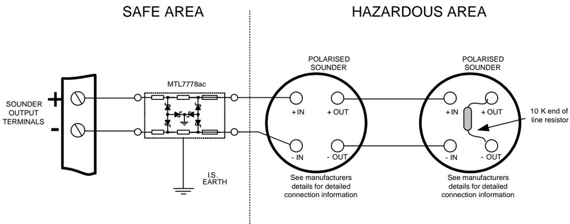
Sounder circuit wiring through an MTL7778ac I.S. barrier
