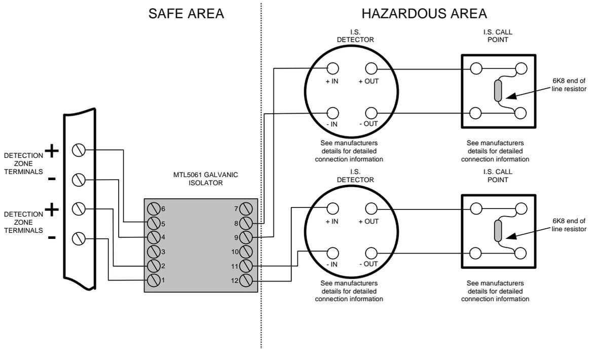
Detection zone wiring through an MTL5061 galvanic isolator
