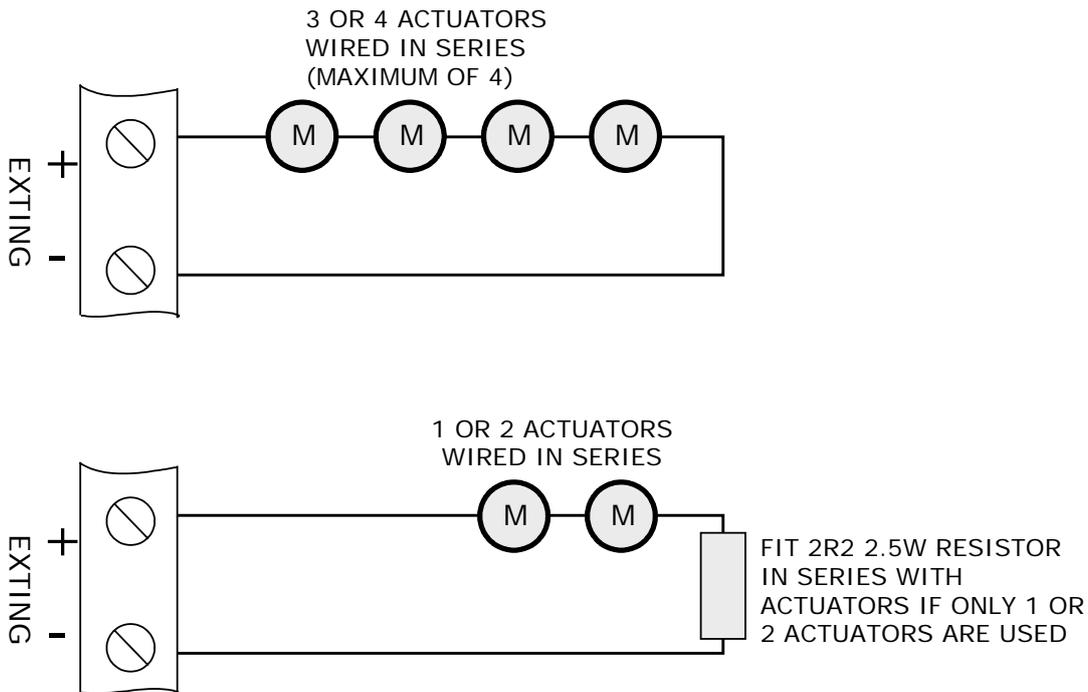
To guarantee firing under all conditions, the total resistance of actuators, monitoring resistor and cable should not exceed 7 ohms.
