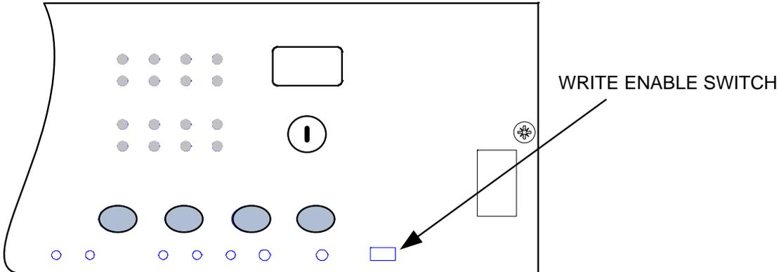
**Access level 3 (Write enable) enable switch location – slide gently to the right to enable**
