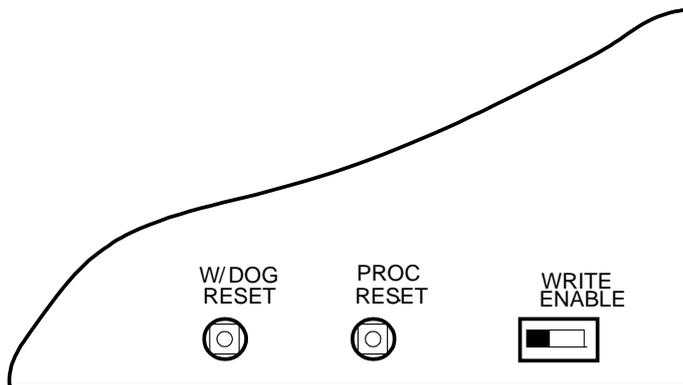
Internal controls on detection part of control panel
